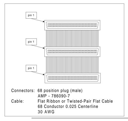
**Connecting Internal and External Wide Devices** The cable assembly for connecting internal wide and external wide SCSI devices is shown below:
